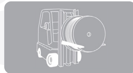
Figure 6: Forklift handling of reels.
