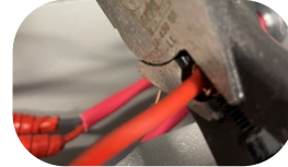
Crimp the bushing twice for secure termination
